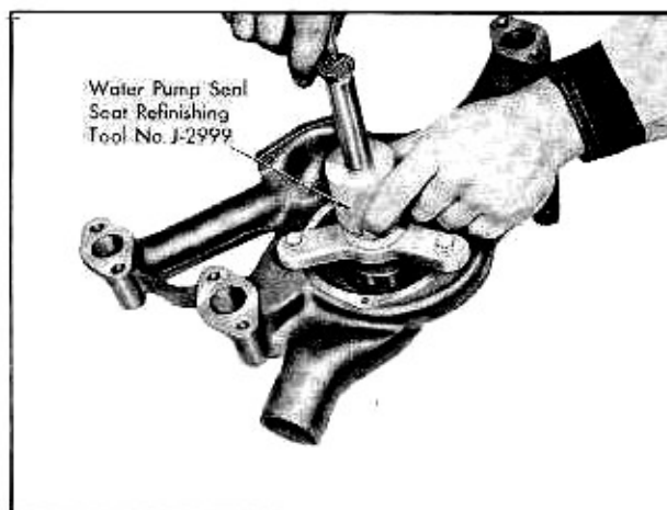
Fig. 13-6 Refinishing Water Pump Seal Seat
